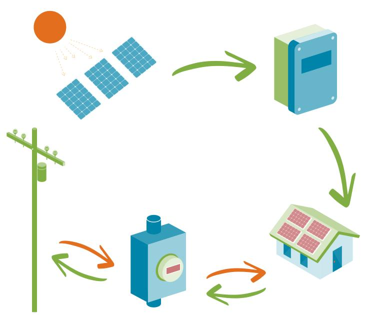
The net meter indicates electricity usage and any excess energy produced is sent back to the grid.
